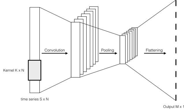
Figure 2.2: Convolutional neural network for time series
