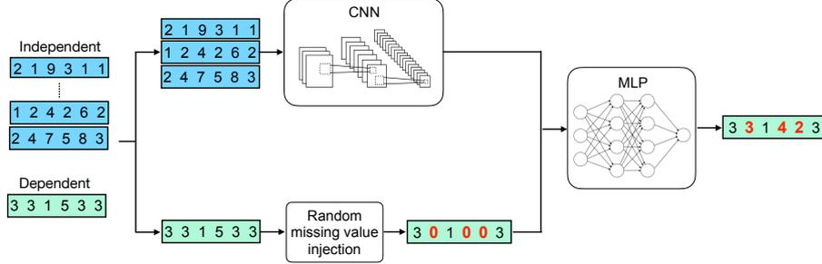
Figure 4.2: Schematic overview of the missing value imputation model
